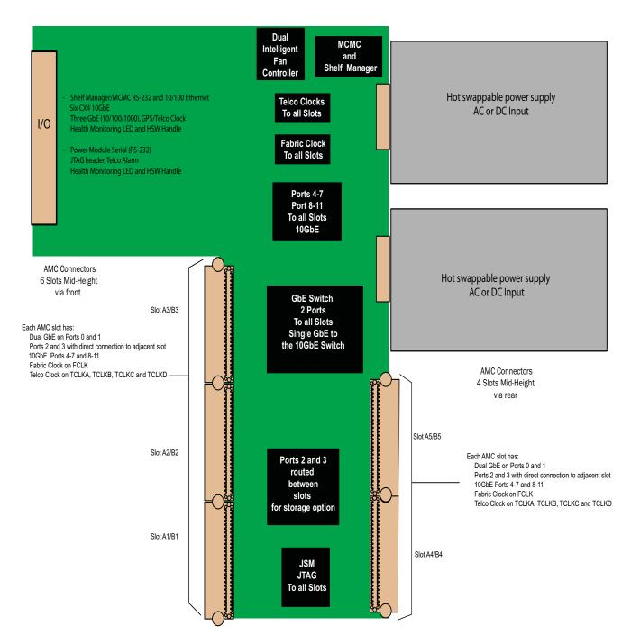
FIGURE 1. VT847 Functional Block Diagram
